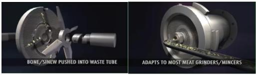
Meat products with Bone / Sinew enters the grinder, the Bone / Sinew collects into the grooves of the holeplate, the flows to the center of the holeplate and exits out of the waste tube. A percentage of Meat products (shown in red) will also follow the same path as the Bone/Sinew. The discharge rate can be regulated by opening or closing of the Ball Valve installed in the waste piping.
